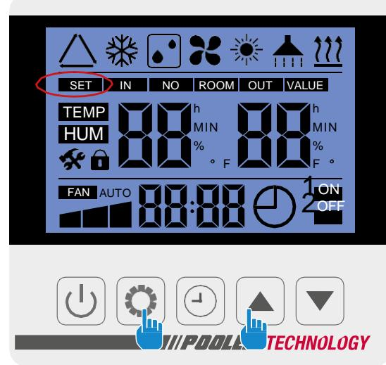
Press + simultaneously for 5s, flashes quickly, the control box is ready to be paired.
