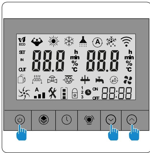
Press + + simultaneously for 5s, flashes quickly, the control unit is ready to be paired.
