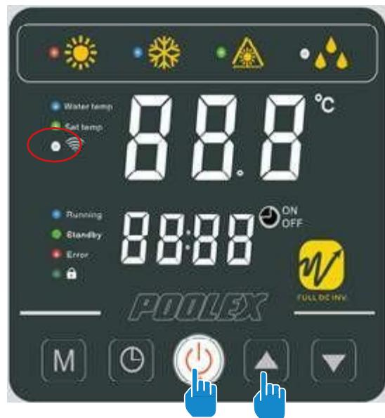
Press + simultaneously for 3s, flashes quickly, the control box is ready to be paired.
